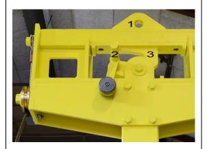
Now "2" and "3" are locked together so you must ensure that "2" is in vertical position and the main wire is taut.
