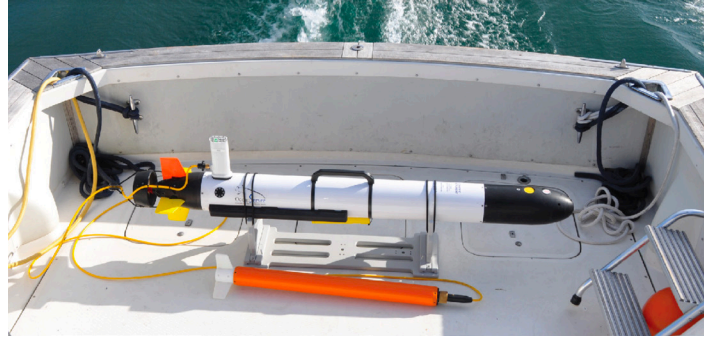
Explorer AUV mag integrated with the Iver2 AUV
